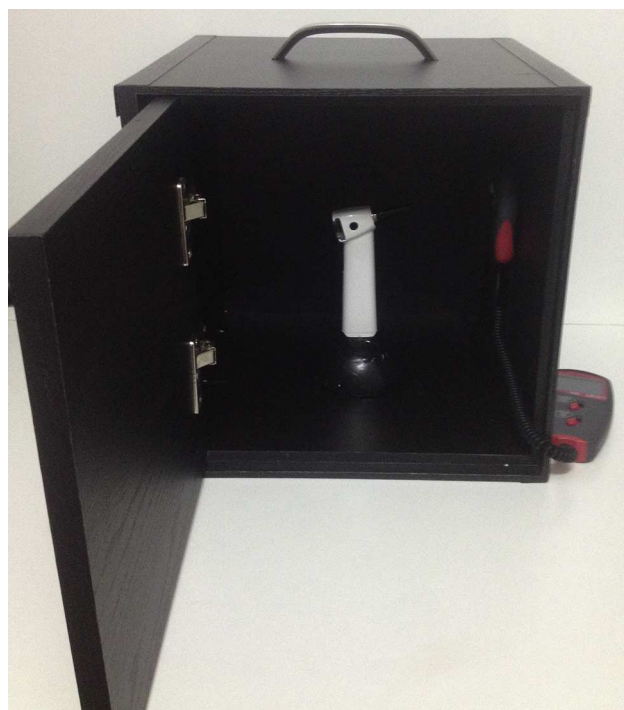
Figure 2 Otoscope fixed at the base at a 4-cm distance and light source directed to the central point of the photometer.
